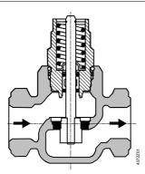
The valve is of the «normally closed» design, where the return spring provides the necessary force to pull the plug against the seat.
